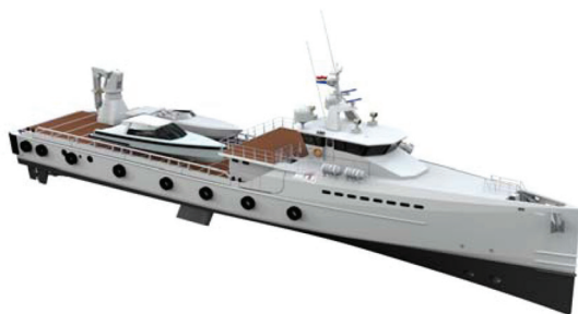
Fig. 4a. The AXE Bow Concept applied as Fast Yacht Support vessel of 50 m length concepts
