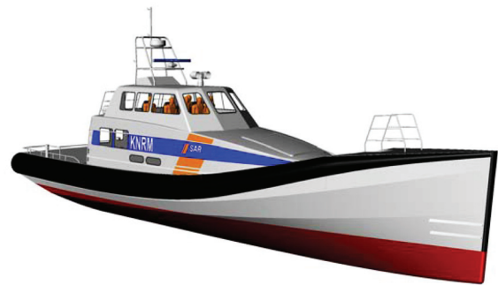
Fig. 9. Proposal for a new SAR vessel for the KNRM with Loa = 21 m and V_s = 35 knots
