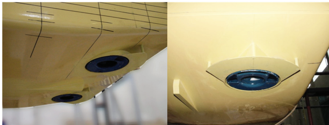
Fig. 3. Detail of ship model ready for self-propulsion test
