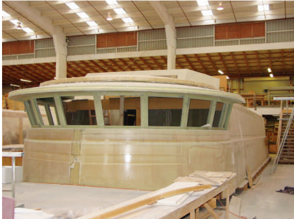
Fig. 3. FRP in superstructure of 33 m HSC yacht
