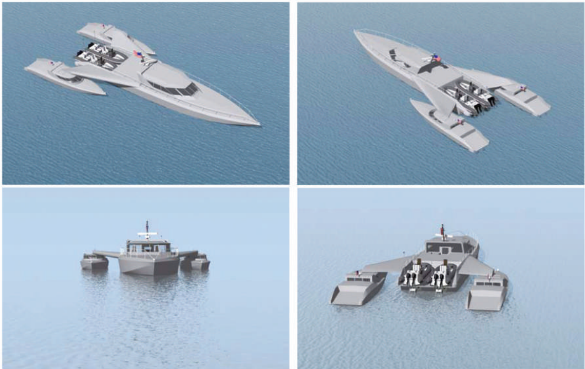
Fig.11. Trimaran concept showing modified wing structure. Position of side-hulls relative to the center-hull has been reduced both transversely and longitudinally based upon transient structural analysis with operation at 50 knots in sea state 3. Center hull is air-transportable in a C17 and has performance specifications similar to existing monohull concepts. Wing-hulls are air-transportable in a C130 and can reach speeds of 82 knots.
