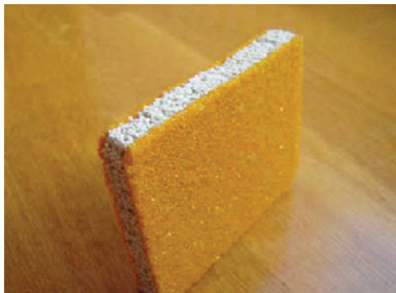
Fig.7b. Building material from recycled composites. Gypsum blocks
