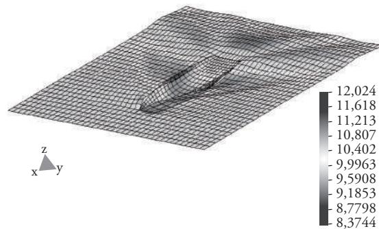
Fig. 1. Representation of runoff on a hull (CFD)
