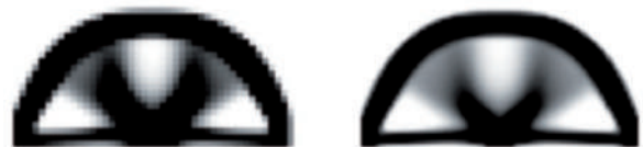
Fig. 3. Topology optimization results for a design domain of (a) 44x22 and (b) 80x40 cellular automata
