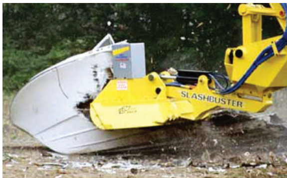
Fig.10. Mechanical cutting of boat hull
