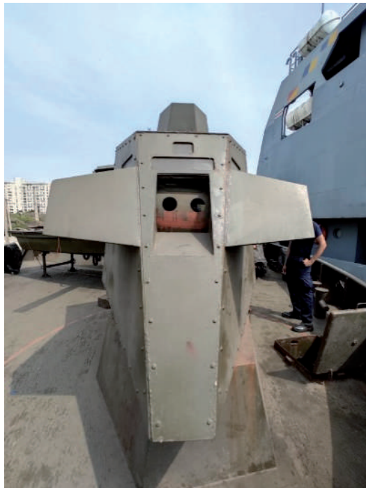
Fig. 8. Forward casemate of A.R.C. unit. JUAN OYOLA.
