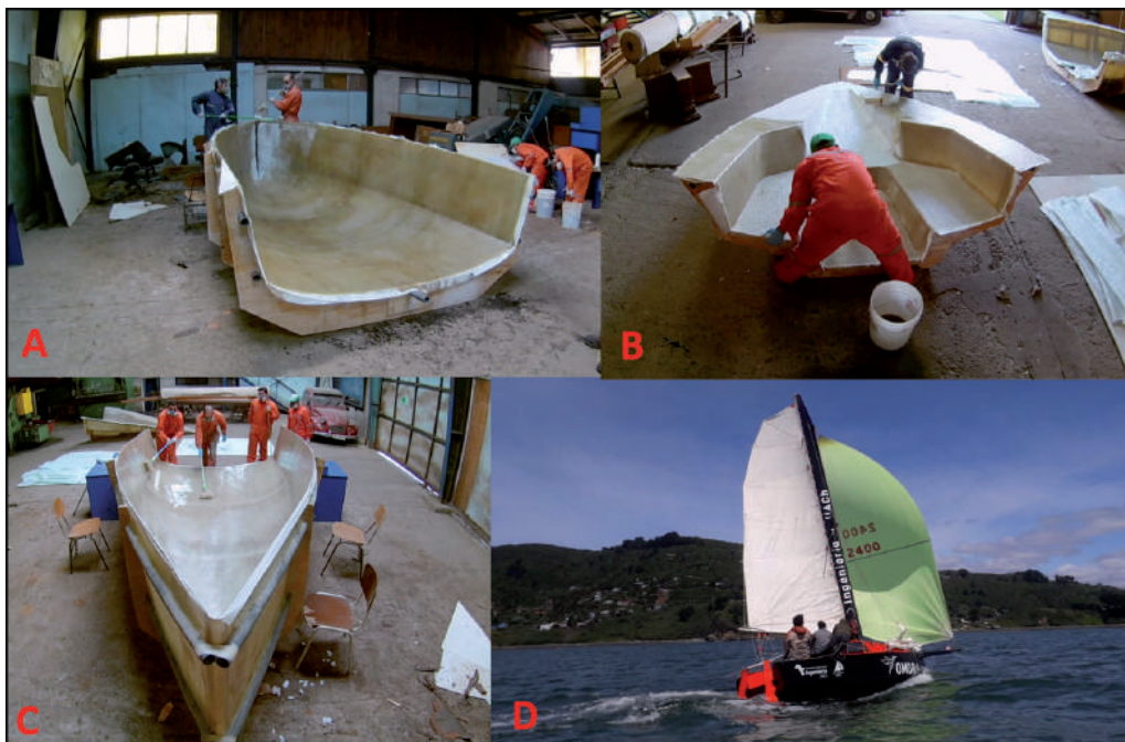
Fig. 1. A and B Manual lamination of hull and superstructure, C Mold lamination and D Finished part (source: A and B): OMORA Project, School of Naval Engineering, Universidad Austral de Chile).
