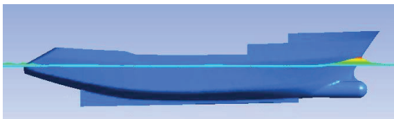
Fig. 7. Wave profile generated by model with bow bulb.
