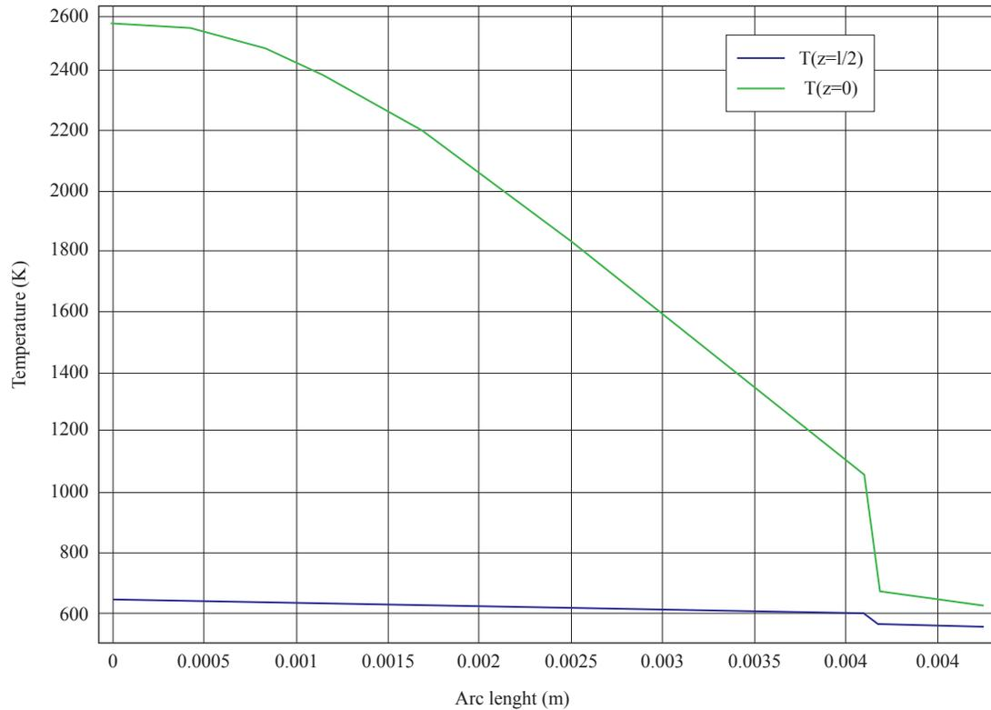
Fig. 12. Temperature in the fuel element (t=60 s).
