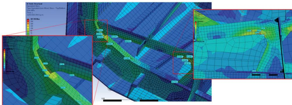
Fig. 12. Equivalent stress over 100 and 120 MPa.
