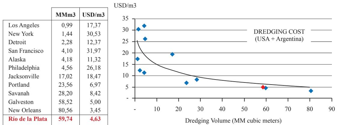
Fig. 6. Dredging Unit Cost Breakdown (LNG).
