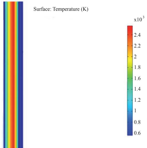
The temperature obtained as a result has a maximum value in the center of the fuel of approximately 2588 K and follows the trend of the typical temperature graph in the radial direction (Fig. 5), as can be seen in Fig.11, obtaining a high value in the fuel, which is decreasing in the direction of the coating. These values depend on the heat source and the radiation that is effected through the gas gap.
