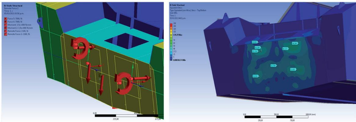
A 45 MPa maximum stress value was reported on transom plate and, therefore, a safety factor of 4.4. It was decided to allow this safety margin taken into consideration aft collision loads, vertical shear forces; as result of outboard motors impacts with objects in the riverbed and future motor updates.
