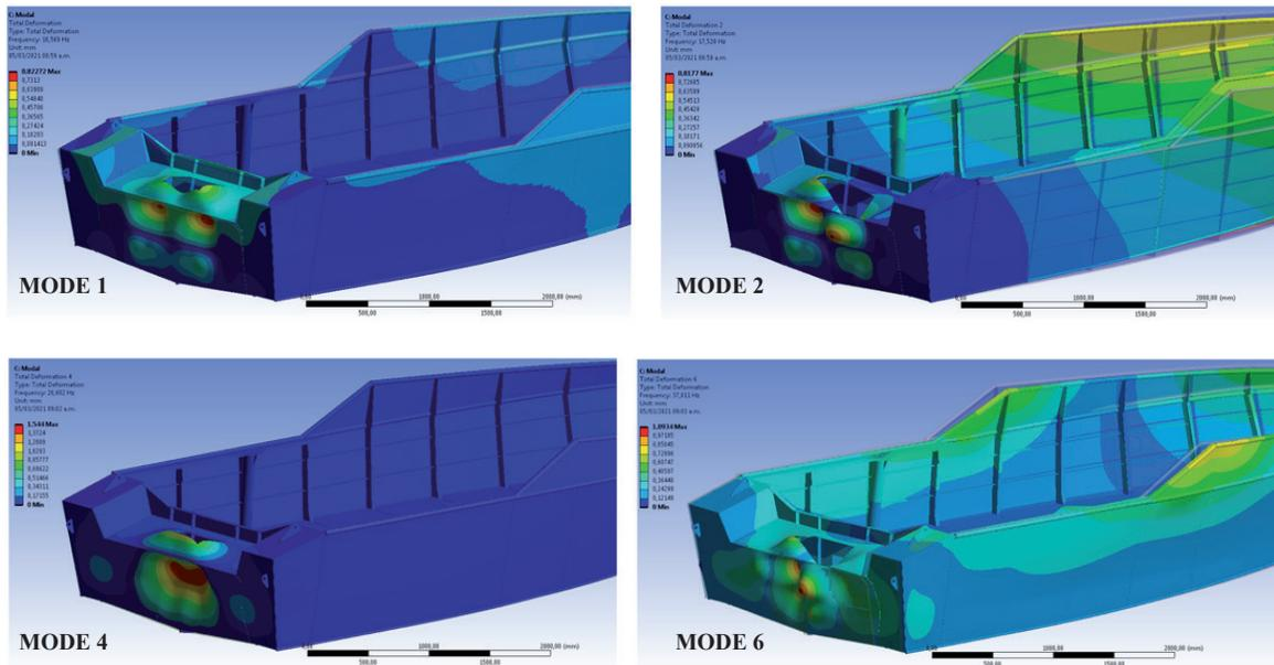
Fig. 20. Buckling load multiplier factor affected zone.
