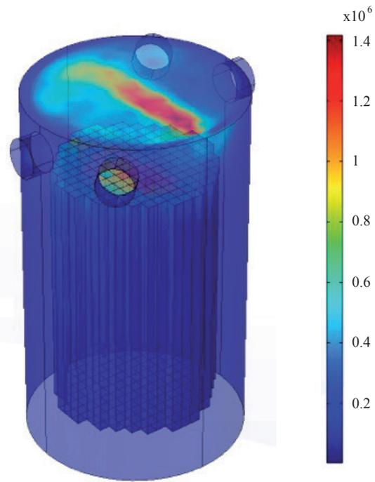
Fig. 19. Radial temperature profile at the rods of the fuel element (t = 60 s).
