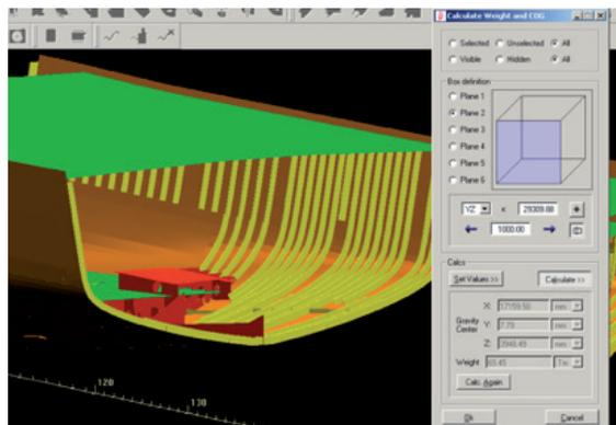
rules as when working in 2D, which means to start with the definition of the continuous elements because this will allow the automatic splitting of the non-continuous elements. However, that sequence could be modified by creating both plates and profiles at different design stages.
