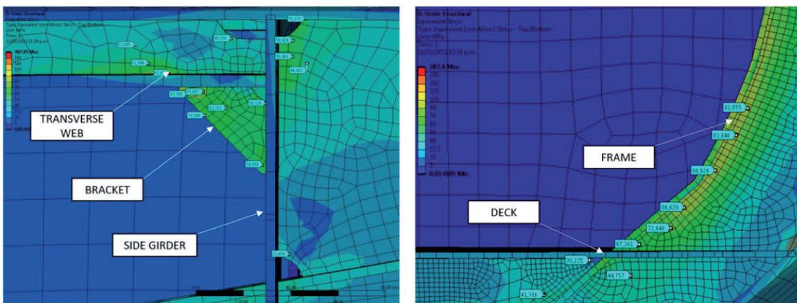
Regarding the frame-deck intersection, typically below 90 MPa stresses were reported in frames due to their curvature near the deck [see Fig.14- right].
