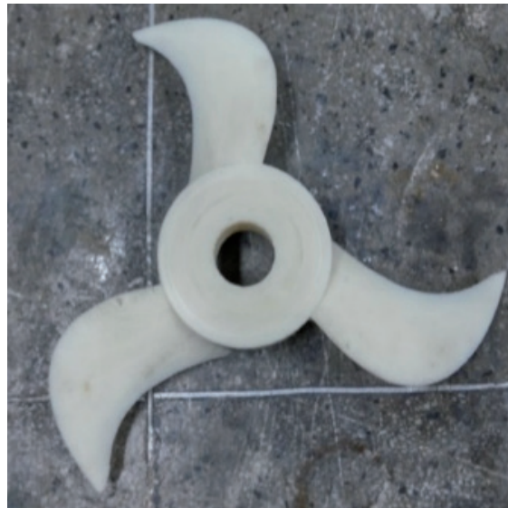
Fig. 8. Speed propeller prototyped by means of additive manufacturing in ABS M30.
