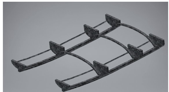
Fig. 19. Structural frame of the catamaran.
