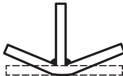
Fig. 1. Angular change due to angular distortion of the fillet weld (Masubuchi, 1980)
