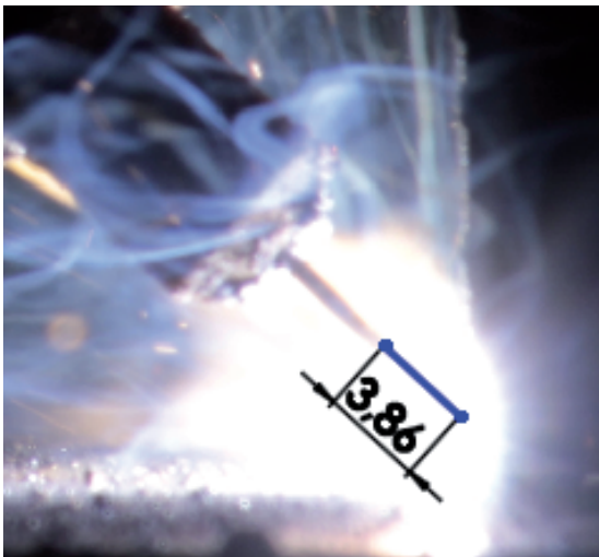
b) Arc length of approximately 3 mm.
