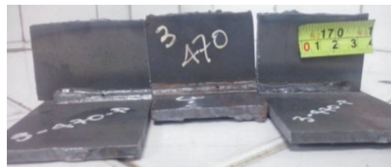
Fig. 7. Weld Coupon WFS=470 \text{ ipm} and LA=3 \text{ mm} in sections for the macro-attacks
