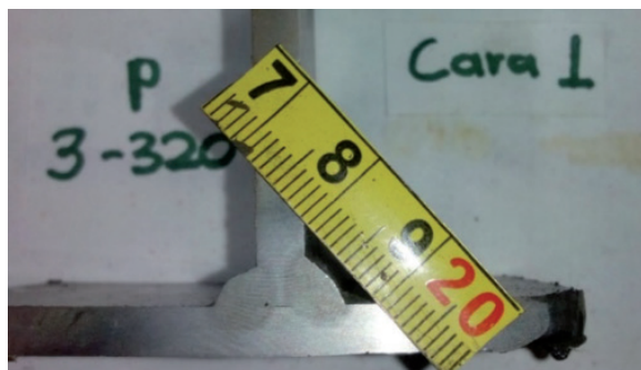
(A) Macro-photography of the weld and replica
