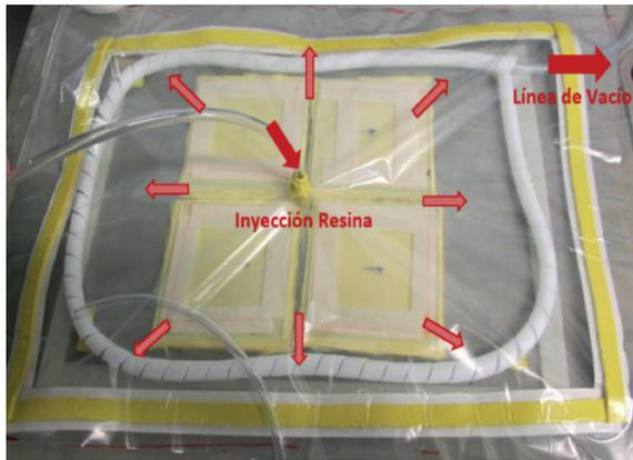
b) Infusion system to 4 samples manufacturing using a central feeding and a peripheral vacuum line: 3 layers of Kevlar + Epoxy Resin
