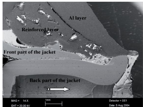
b) Detail of the projectile output: compressed and high-deformed layers, mixing regions, high deformation and geometrical changes of the peeling cap
