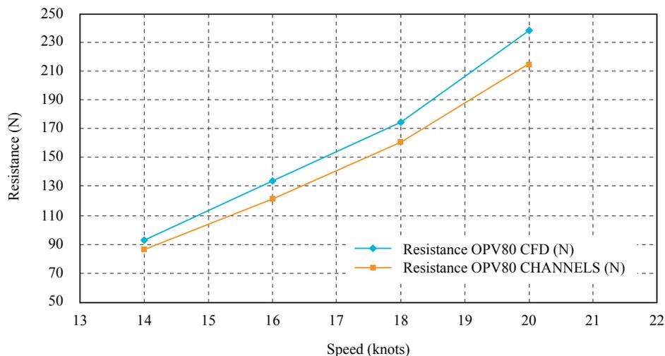
Table 4. OPV 80-channel and OPV80-CFD hull advance resistance values
