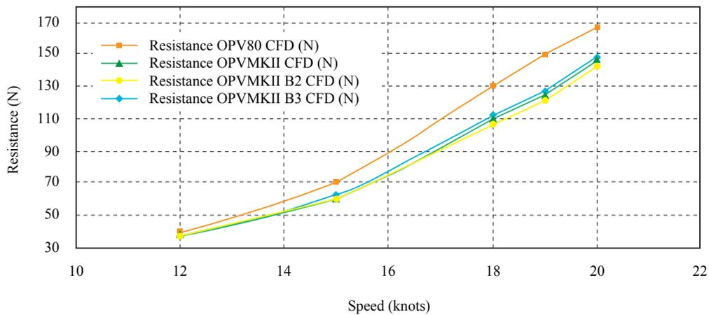
decrease in the resistance to the advance in the hull is closed, however there are considerations that can influence the use of one bulb and another, as is the case of the pitch of the vessel and the percentage of time in the life cycle that the ship will operate at certain speeds.
