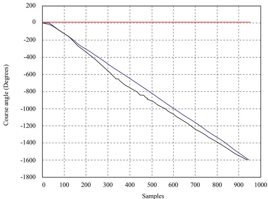
Fig. 4. Comparison between the output of the second-order (discontinuous) Nomoto model and the actual heading angle with the validation data
