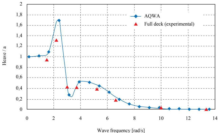
Fig. 20. Heave RAO of the reduced vs. simulated model (AQWA) in the direction of 90°
