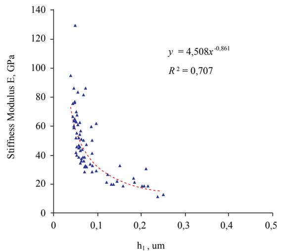
b) Sample B1: Glass Fibers + Epoxy Resin
