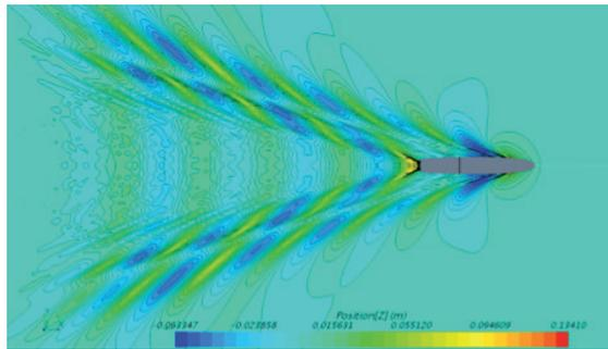
Fig. 18. View of hull flow lines OPVMKII B1
