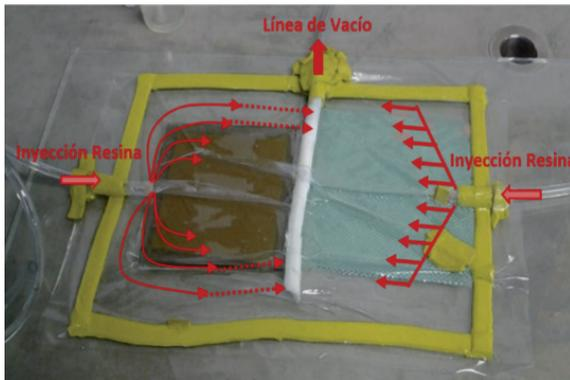
a) (left) 3 layers of Kevlar + Epoxy Resin; (right) 7 Layers of E-Glass fibers + Epoxy Resin
