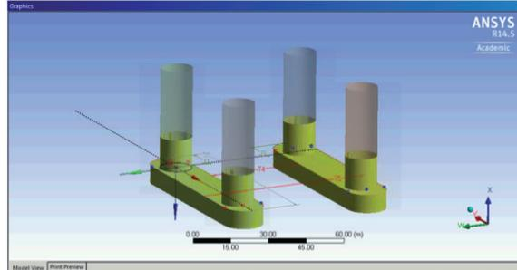
The experimental response of natural frequency obtained by the model is equivalent to approximately 0.4 Hz according to the analytical calculations ( $2.52 \text{ Rad / s} \approx 0.401 \text{ Hz}$ ) which represents concordance with the constructed physical model.
