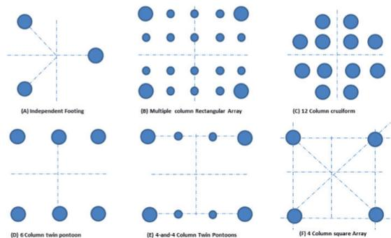
Fig. 4. Arrangement of pontoons in semi-submersibles [CHAKRABARTI, 2005]
