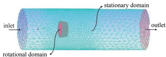
Calculations are carried out by the “Fluent software” to solve the three-dimensional viscous incompressible flow. The steady state pressure-based solver in a segregated mode was implemented using the MRF technique.
