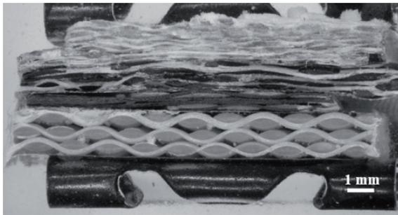
a) Laminate samples extracted for optical inspection and nanoindentation tests
