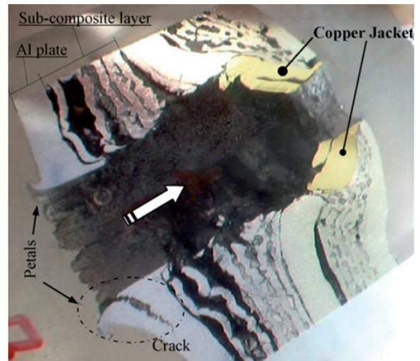
a) General view showing some failure mechanisms as petalling, swelling, delamination of layers, high strained regions by compression and shear, melting welding, bending and bulging
