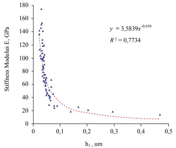
a) Sample B3: Carbon Fibers + Epoxy Resin
