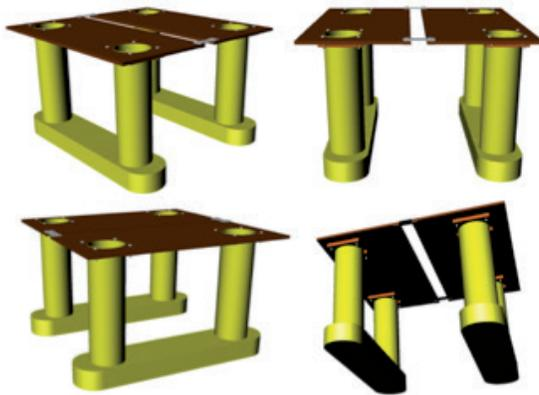
The pontoons and the columns were constructed with PVC and the deck with compensated wood. The use of epoxy resin and PVC reinforcements was crucial to give rigidity to the structure and guarantee the water tightness of the model once it is floating in the water (see Fig. 12).
