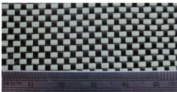
d) Mixed woven fabric: Kevlar and Carbon Fibers, density: 185 g/m<sup>2</sup>
