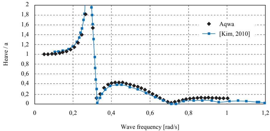
In Figs. 19 and 20 the constructed model validates the hydrodynamic behavior obtained in computational simulation, especially in relation to natural frequency.
