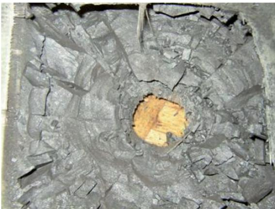
b) Biomorphic ceramic (RBS) impacted by 7.62x63mm AP-M2 projectile
