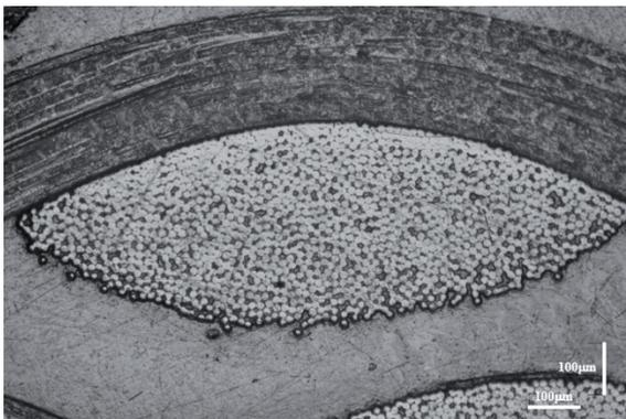
c) Detail of branches of Kevlar fibers (optical microscopy): longitudinal and cross views of fibers
