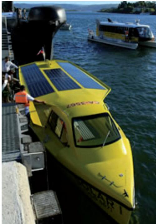
A roof covered with photovoltaic panels has been designed, see Fig. 10, normally placing a heavy weight on deck that could be a problem for the stability of the boat. However, this moderate weight is amply compensated by the greater weight of the battery bank, conveniently located as low as possible. The panels continually recharge the
