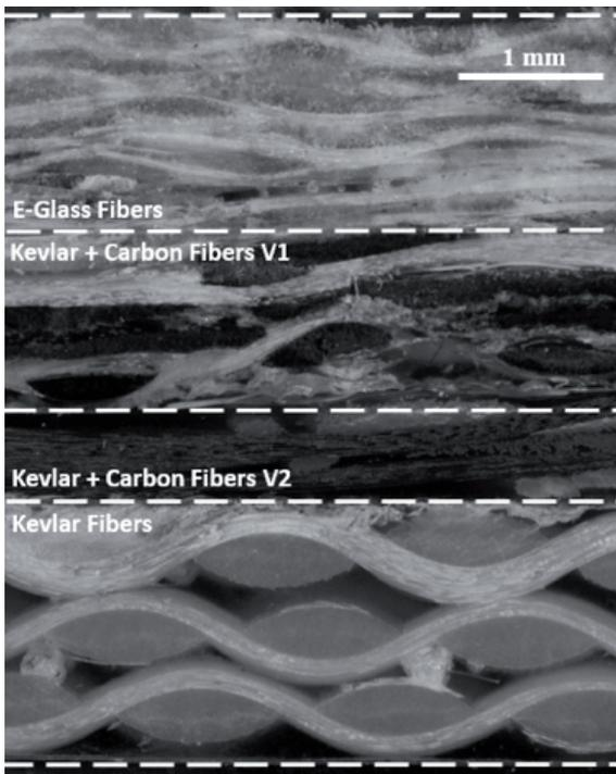
b) Stereo micrograph of a set of 4 samples of different configurations
