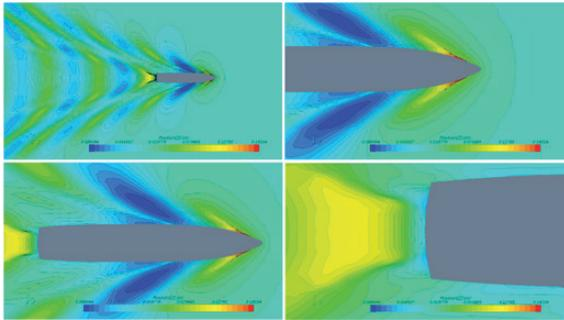
Fig. 9. Views and approaches of pressure distribution in the hull of the OPV 80 vessel
