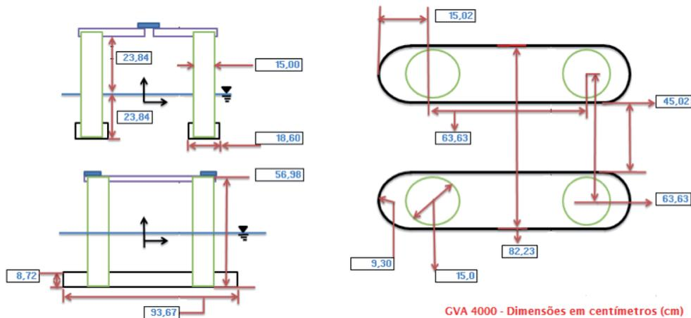
Considering the physical characteristics of the tank, a scale factor of the 1:86 model was established.
