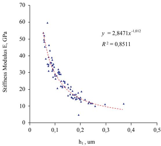
c) Sample B8: Kevlar Fibers + Epoxy Resin
