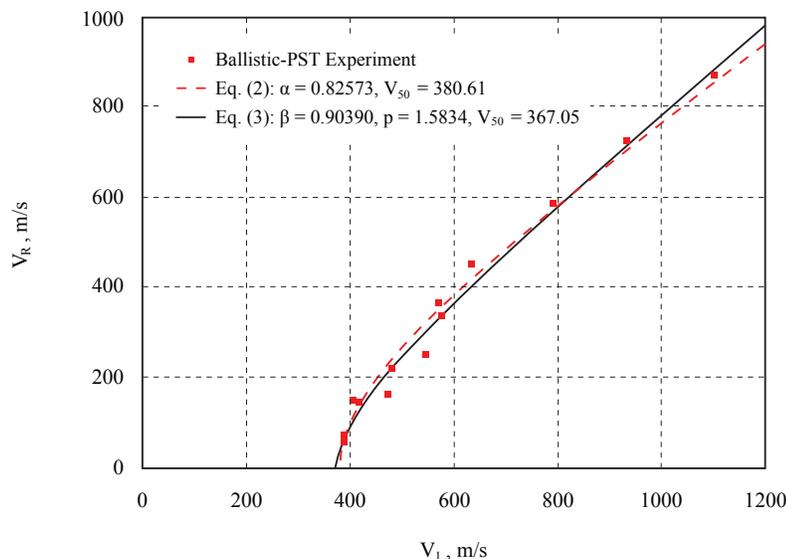
penetration model and a method to determine the ballistic limit  $V_{50}$  for laminar composite materials [30-32]. We currently are working to enhance the applicability of this model to laminar composite materials reinforced with hard ceramic particles.
