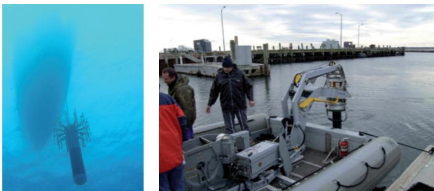
On the other hand, it is important to highlight the USV Darco, which is a USV with a multi-configuration for Antisubmarine warfare. This USV can be equipped with torpedo launchers, depth sounder, Active Source and towed Sonar. The USV Darco is a development proposed by the company General Dynamics that seeks to supply this type of USV for the Littoral Combat Ship - LCS type ships of the US Navy. [5]
