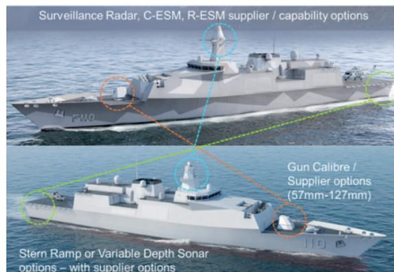
For a platform design to be attractive to a number of Navies it needs to have the flexibility to incorporate a variety of combat system equipments from different suppliers, all without increasing the risk within the design or the cost of each individual programme.
