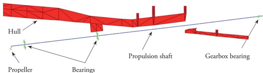
Fig. 6. Propulsion line drawing.
