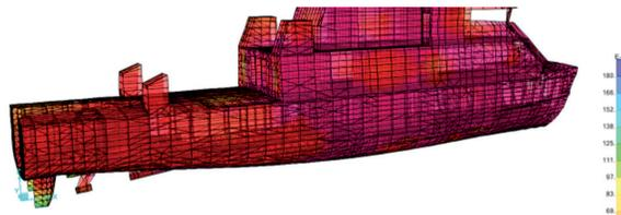
Deformation was estimated at all nodes in the model, for each load condition. Figs. 16, 17, 18 and 19 graphically show deformation results.
