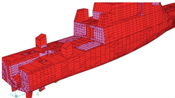
Fig. 2. FEM interior view: Engine room.
