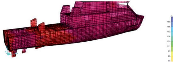
Fig. 17. Deformation (mm) at 29.73Hz condition.
