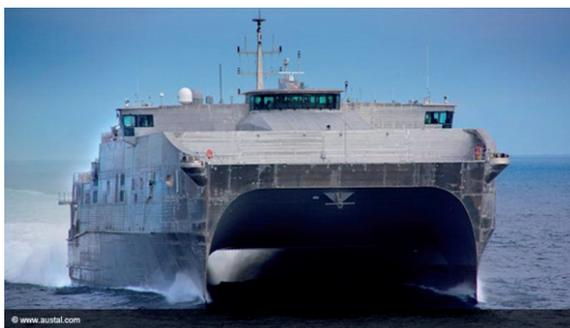
Currently, companies such as Austal and Lockheed Navy, leading the military application vessel design and fabrication sector, mainly for the U.S. Navy, have completely revolutionized these types of vessels, replacing the traditional structure with a revolutionary structure based in multihull solutions, with the purpose of achieving speeds that exceed 45 knots, larger flight decks for helicopters, as well as a considerable increase of internal spaces.
