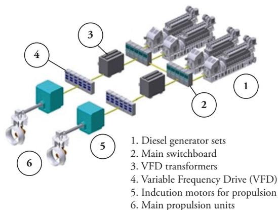
The prime movers drive the electric generator producing electrical energy. The electric power is distributed and transmitted to the propulsion motors which provide torque to the propulsion units. The electric motors are driven by Variable Frequency Drives (VFD) which are feed by transformers.
