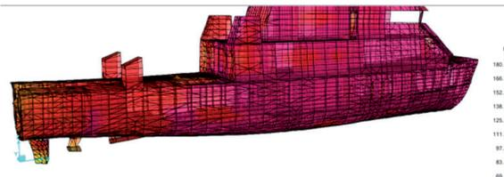
Tables 14 and 15 show vibration speed values by sector for each condition, calculated from the deformation found with the FEM. Most vibration levels do not exceed the limits set by the rules, except the aft bulkhead on upper deck at 2000 RPM, where the limit is 6 mm/s.
