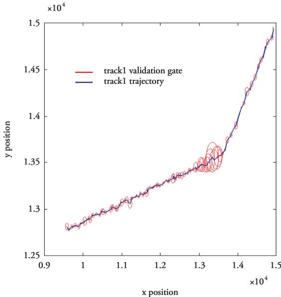
As a result, the validation area was expended because of increasing of difference between measured position and predicted position by unexpected turn at 20 second.
