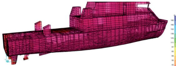
Fig. 18. Deformation (mm) at 37.77 Hz condition.
