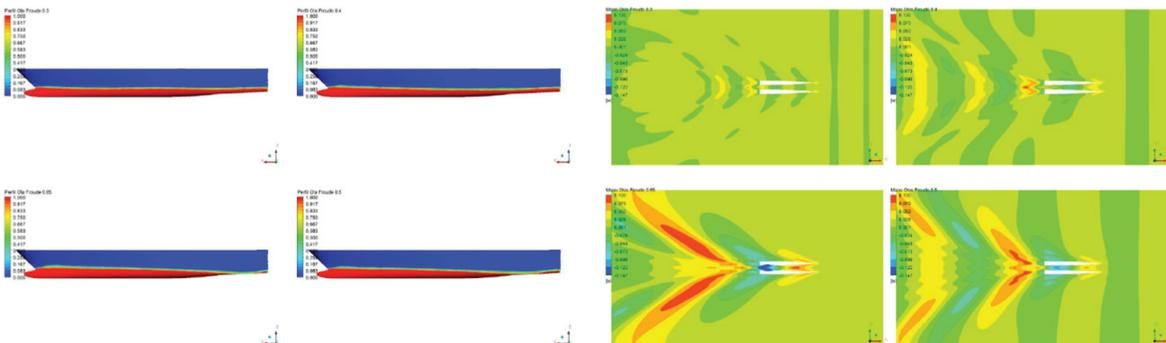
displacement of the original bottom. Analogously, once the bottom's buoyancy is studied, and the  $C_{cf}$  index is obtained, the application may assess the convenience of introducing modifications to it by adequate sleeve distribution. The lesser the  $C_{cf}$  index the less resistance to advance of the bottom.
