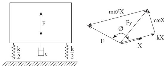
Transmissibility is the relationship between the perturbing force and the transmitted force to the foundation and depends especially of the connection stiffness between the engine and the boat structure. For this study, flexible rubber mounts had been used.
