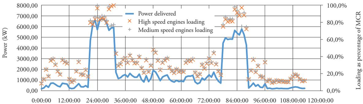
Fig. 14. Performance Analysis for Arrangement 3.
