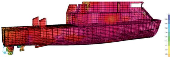
Fig. 20. Deformation (mm) at 43.86 Hz condition (reinforced bulkhead at upper deck)
