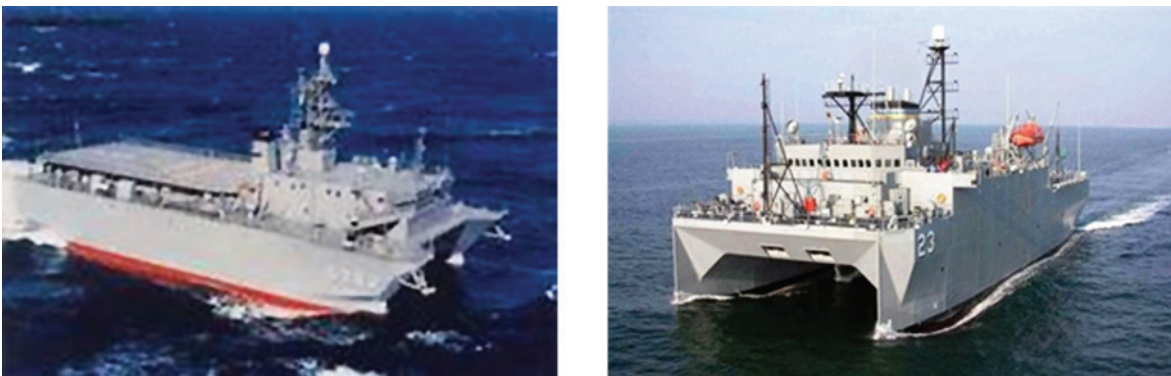
Fig. 9. SWATH Hull Forms
