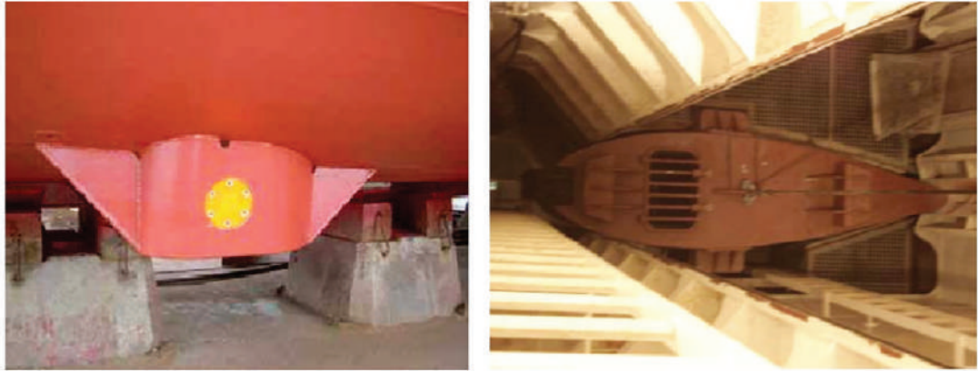
Fig. 2. Retractable Keel and Transducer
