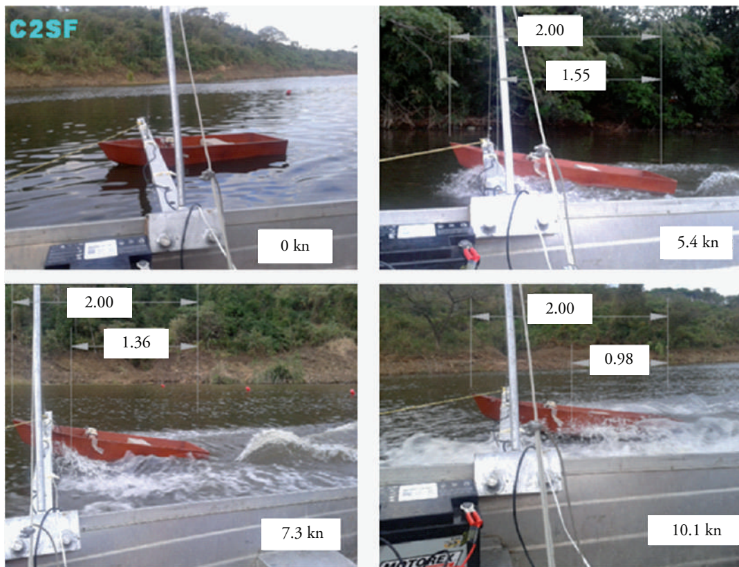
Fig. 4. Tests with no flaps in load condition 2
