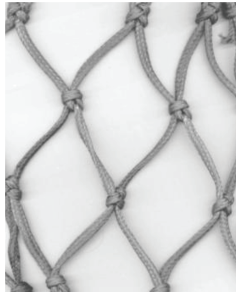
Fig. 1. Weave of a polyethylene net
