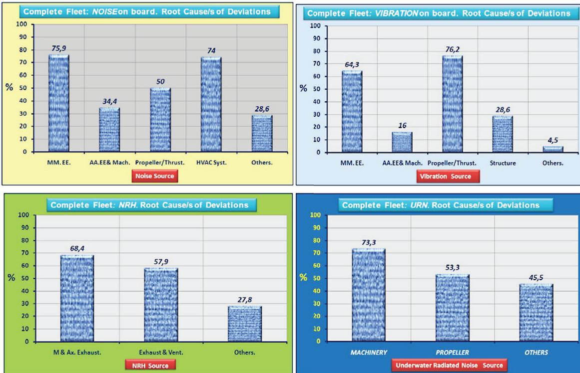
the deviations detected in the noise radiated by the vessel into the water with regard to the preliminary URN targeted limits. This approach is consistent enough with the experience documented at Glacier Bay, mainly related to passenger vessels.
