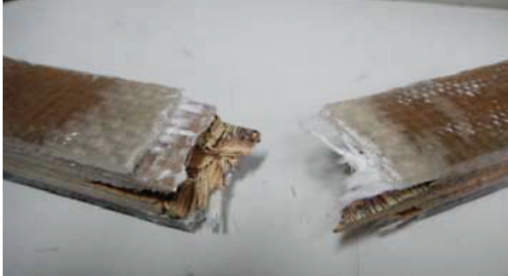
Fig. 2. Sandwich material after traction
