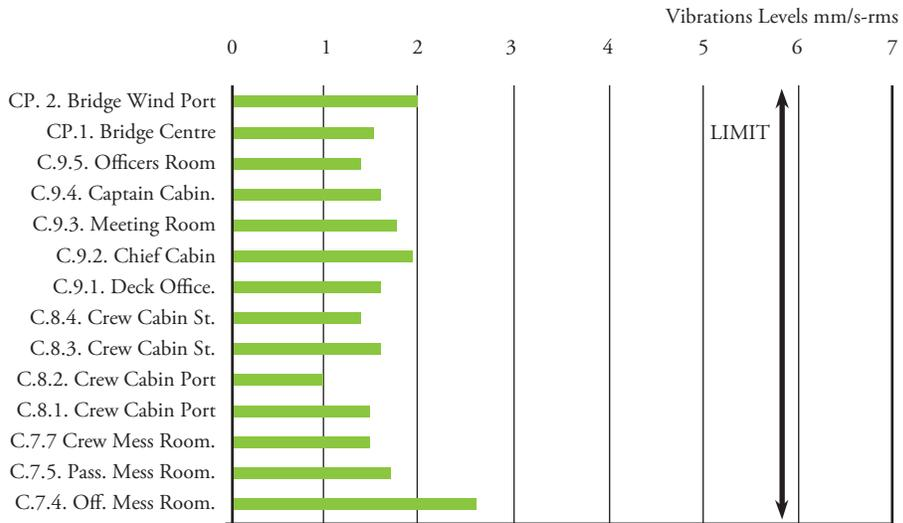
Fig. 18. Noise Levels obtained at different Locations
