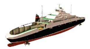
Principal dimensions and propulsion units:  $L_{OA} = 129.80 m$   $L_{pp} = 122.40 m$  LWL = 128.87 m BOA = 18.70 m  $T_{Max} = 4.10 m$ Disp. = 3899 t
