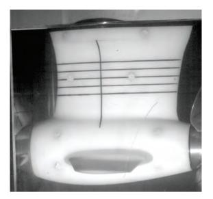
Fig. 15. New Design – Cavitation Test
