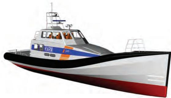
From an extensive series of experiments carried out with a model of this new design and a model of the existing boat in the towing tank, it has been demonstrated that a considerable improvement in the head seas conditions has been achieved with the new concept, without any loss of performance under following and stern quartering conditions.
