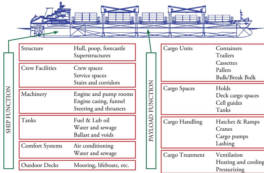
are those related to the transport of passengers and cargo safely from port to port with certain speed, namely the ship as a system, consisting of ship's hull (main and superstructure), facilities of crew, navigation control (bridge), machinery, tanks (fuel and lubrication oil, water and sewage, ballast and voids), comfort systems (air conditioning, water and sewage, electrical), mooring and life-saving equipment, etc. (Fig. 1).
