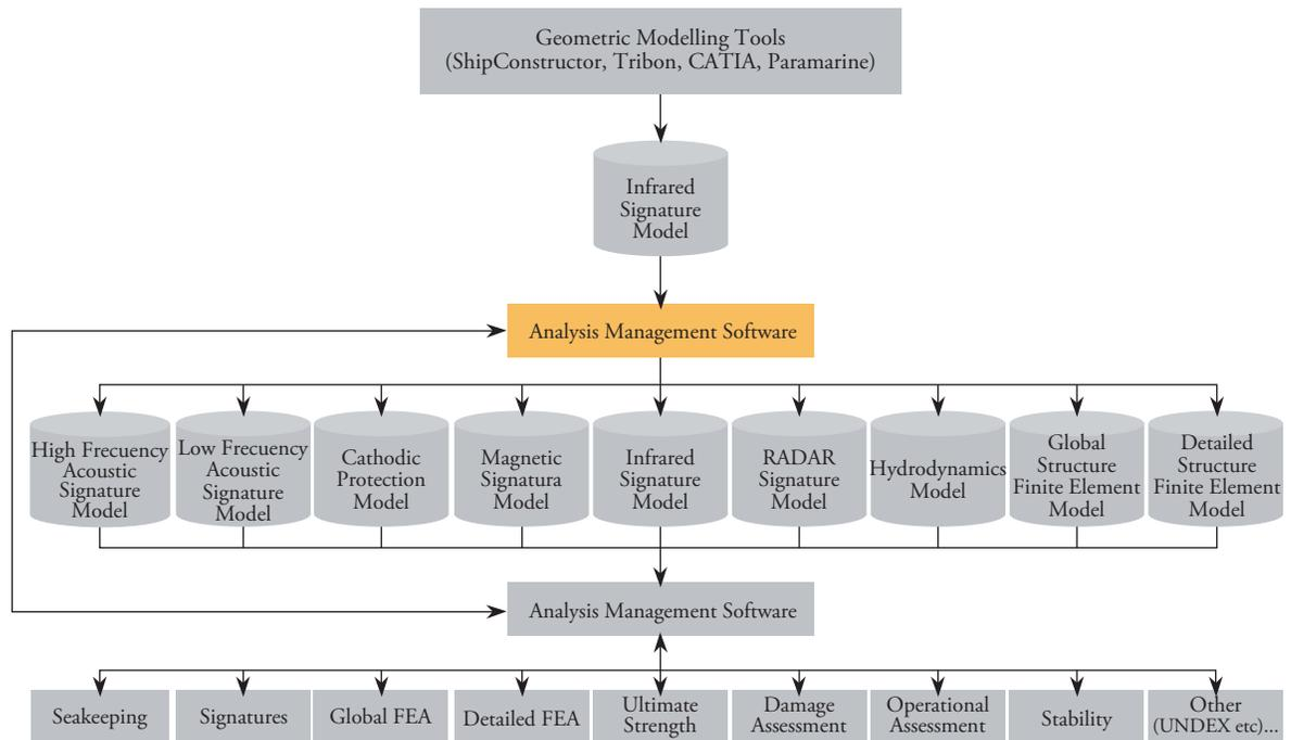
and within budget, able to perform as required and predicted. An example of such an integrated toolset is shown in Fig. 12.
