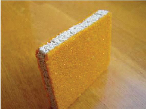
Fig.7b. Building material from recycled composites.
