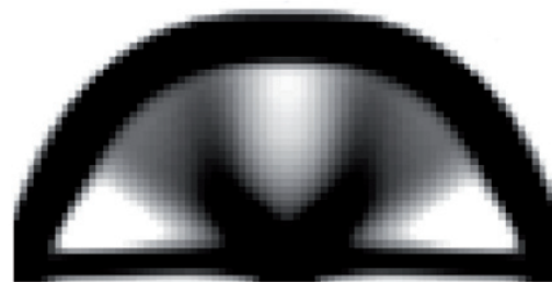
Fig. 6. Topology optimized structure with M/M_0 < 0.4
