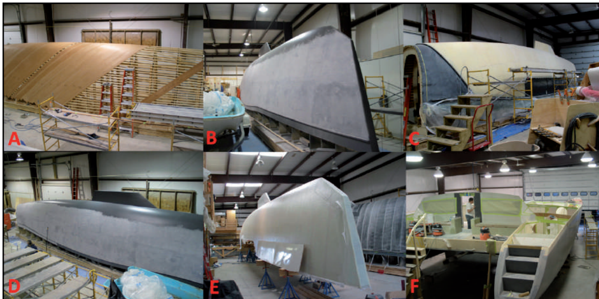
Fig. 5. ONE-OFF construction method - A- base matrix construction, B- inner skin lamination, C- core lamination, D and E- outer skin lamination and F- finished parts.
