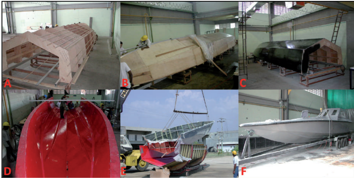
Fig. 5. ONE-OFF construction method - A- base matrix construction, B- inner skin lamination, C- core lamination, D and E- outer skin lamination and F- finished parts.
