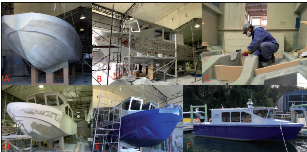
Fig. 14. Finishing: A -hull turn, B -finishing and caulking, C -engine room structure lamination, D -surface finishing, E -hull painting, and F -finished vessel.
