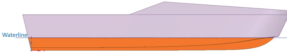
SpaceClaim 2022 software. Only external hull surfaces were included. These hull surfaces are divided by the waterline [see Fig. 3].
