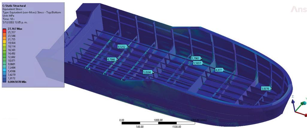
At head seas conditions, the effect of hull's hydrodynamic pressures on the structural arrangement stress levels decreases in comparison with others load cases and this behavior is consistent with the pressure levels showed in Fig. 9. Higher stresses are reported in the bottom – side assembling [see Fig. 22 & Fig. 23].
