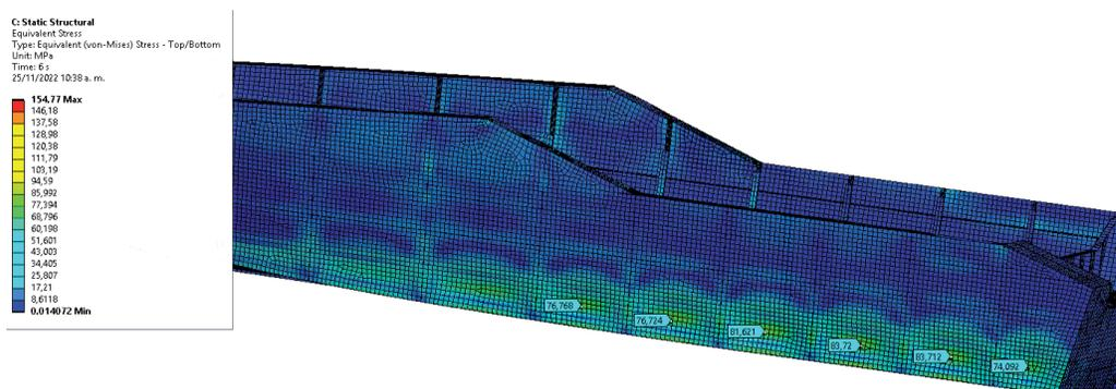
Fig. 18. Stress distribution in the frames with beam seas.
