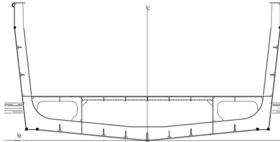
The deck is composed of a AW 5083 H321 plate and seven flat-bar longitudinal stiffeners. This deck is transversally supported by profiles deck beams and bulkheads and longitudinally supported by two side girders.
