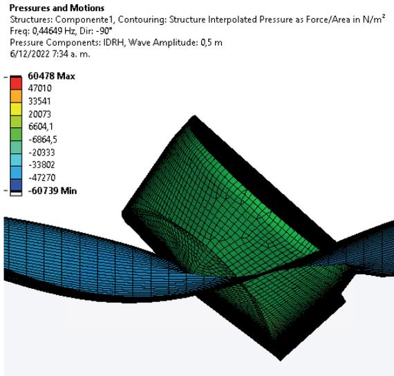
The calculation of hydrodynamic wave pressures according to classification rules such as ABS in [2] and LR in [14] at head sea conditions and also neglecting slamming pressure factors, present the both bottom pressures estimations as two times higher than obtained with the software [see table 7]. Additionally, because the time-dependent nature of loads and the hydro-elastic response of the structure under slamming conditions, the
