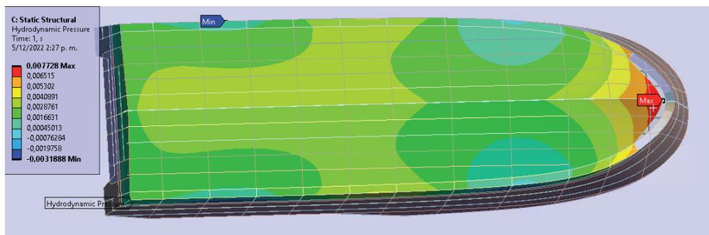
Fig. 26. Stress levels at aft section of the boat.
