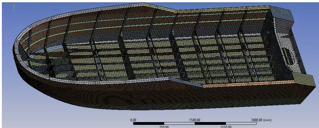
avoid built-in stresses so the reaction forces in the boundaries are to be minimized [4]. ANSYS Inertia relief option allows to exactly balance the force differences on the supports creating a state of static equilibrium. Two of these fixation points were applied at transom intersecting the main deck at portside and starboard, and the last one, in the bow centerline intersecting waterline.
