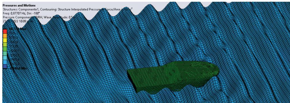
Fig. 11. Imported hydrodynamic pressures at 0.44 Hz and 180° heading – head seas condition.
