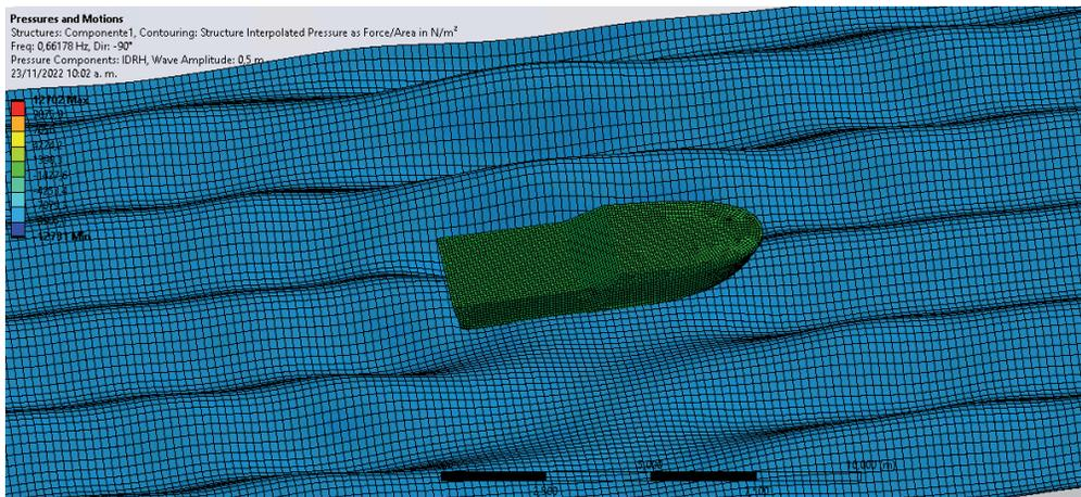
Fig. 13. Imported hydrodynamic pressures at 0.44 Hz and 90° heading – beam seas condition.
