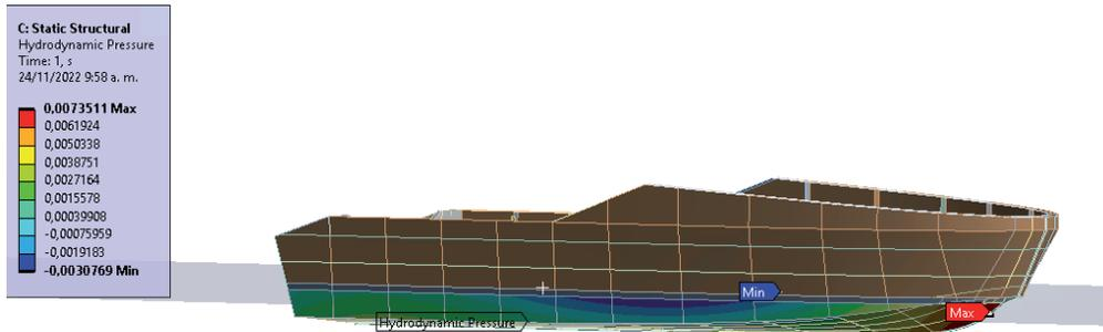
Fig. 12. Pressures and motions at 0.66 Hz and 90° heading– beam seas condition.
