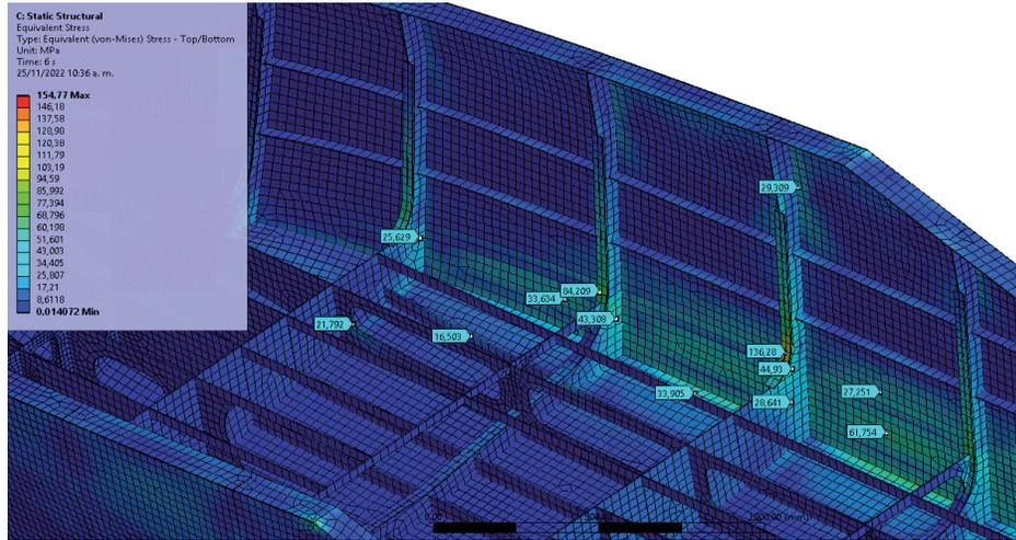
Fig. 19. Stress distribution over the deck.
