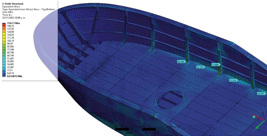
Fig. 20. Stress distribution above 20 MPa with a 120° heading..
