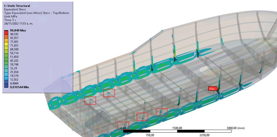
Fig. 21. Stress distribution in side's plates and internals.
