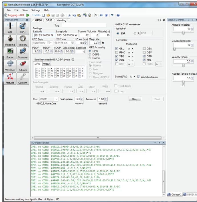
Fig. 5. Serial data reading application [11].
