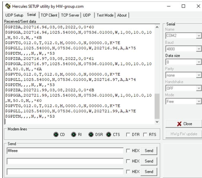
stabilization data. This test allowed validating the frames that are processed and generated by the DDU prototype, from the information coming from the sensors and NDP systems, which is required by the ship's weapon system.
