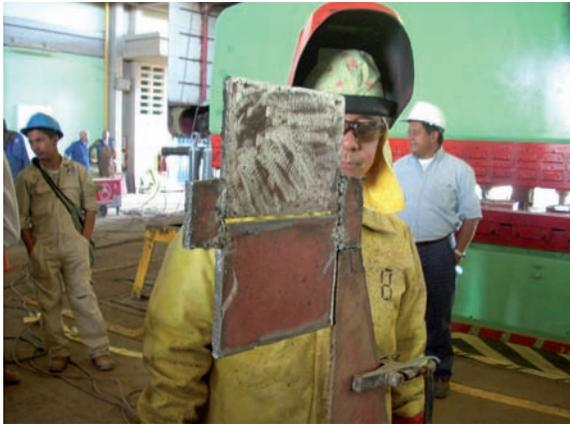
Fig. 6. Test coupon of naval steel of the type ASTM A131 Gr A, steel manufactured in 2008 and one from 1972.
