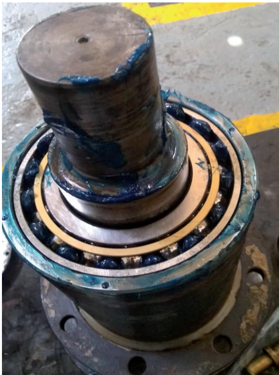
Fig. 8. Lower jib crane support after maintenance.
