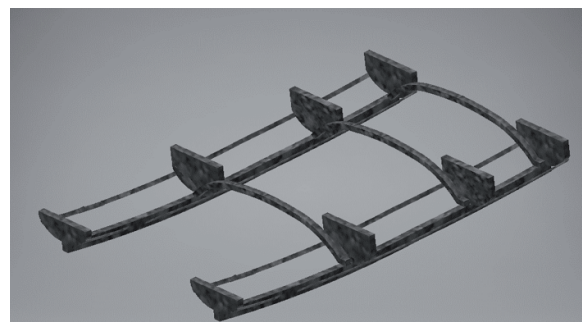
Fig. 19. Structural frame of the catamaran.
