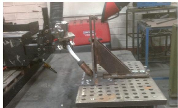
(C) Pistol and coupon arrangement in 2F
