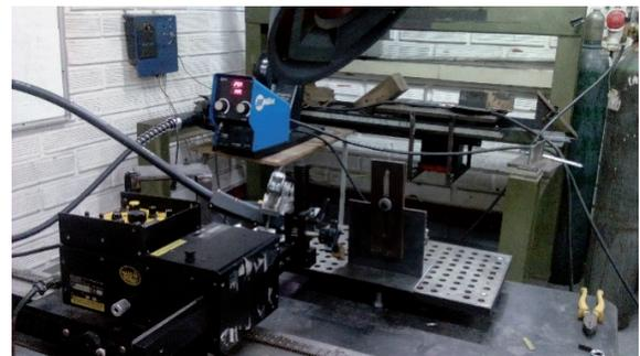
(B) Bug-O automated equipment and test coupon
