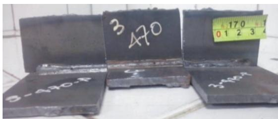
Fig. 8 (A) presents the macro-photograph of the welding applied with  $WFS=320 \text{ ipm}$ ,  $LA=3 \text{ mm}$  and  $23.8 \text{ V}$  (left fillet) and that of its replica (right fillet), respectively. Fig. 8 (B) shows the image processed in SOLIDWORKS with the fillet estimated dimensions.
