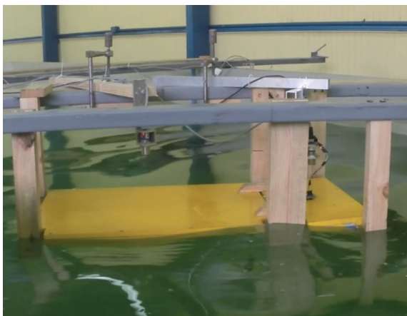
Fig. 13a. Wave tests typical condition given by fetch. H1 / 3 = 0.52 \text{ m} T = 2.99
