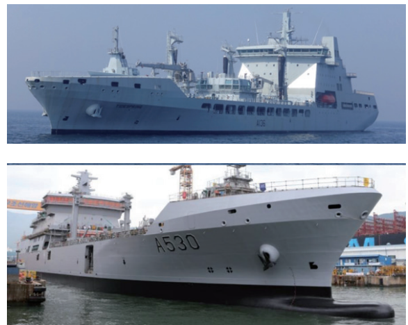
Fig. 2. (top) BMT Aegir® design for the UK Tide Class designed to Lloyds Register naval rules. (below) BMT Aegir® design for the Royal Norwegian Navy designed to DNV naval rules
