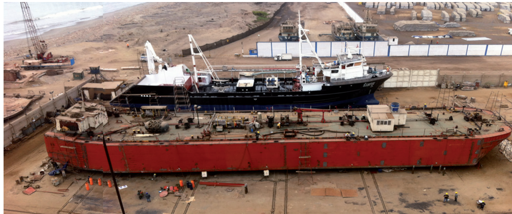
Fig. 22. View Barge "ANTU" in final stages of work. Behind the fishing vessel "SIMON" after lengthening it.
