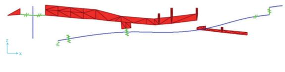
Fig. 12. Second vibration mode 29.73 Hz.
