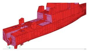
Fig. 2. FEM interior view: Engine room.
