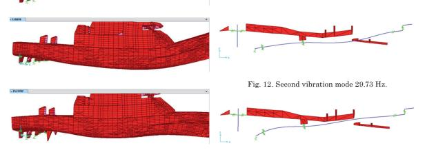
Propulsion line natural frequencies are within the working range and forced analysis should be considered to check the structures resistance and whether the proposed vibration levels standards are met.
